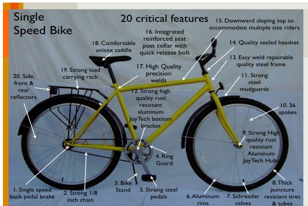
Figure 2: Critical features of a commuter bicycle
