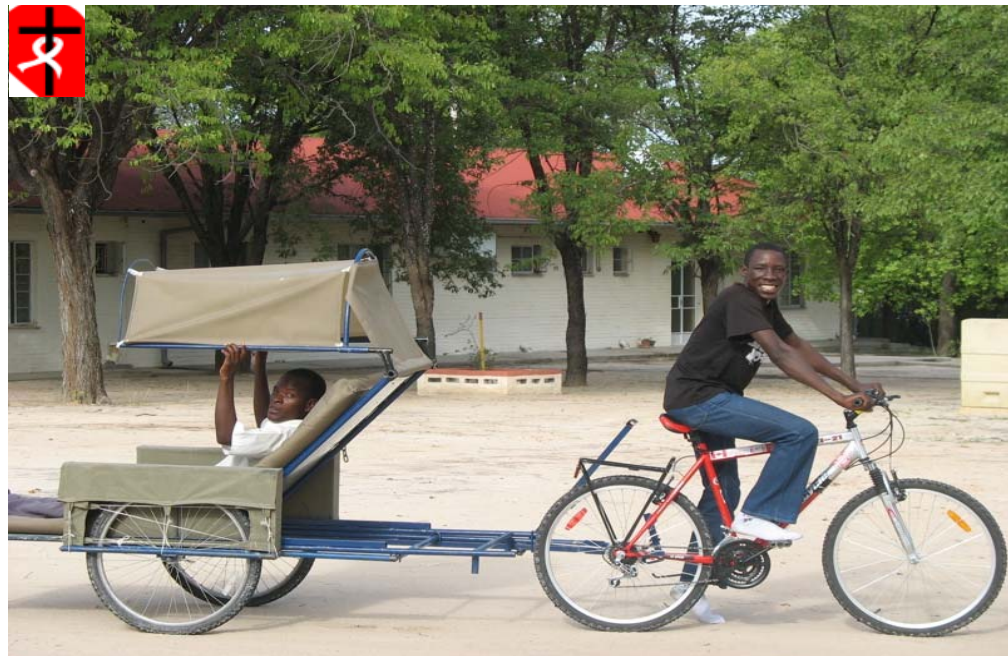
Figure 13: Bicycle trailer for the transportation of patients
